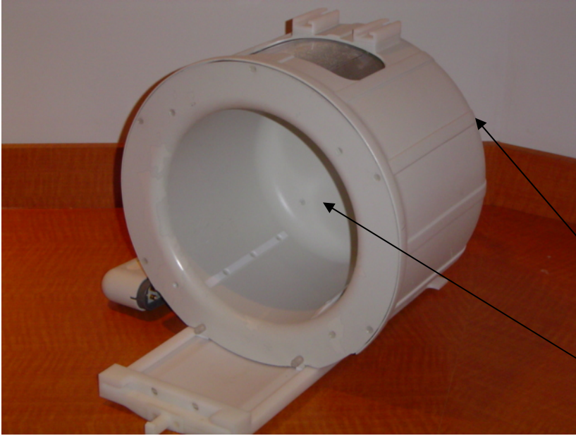
Figure 1. 7T Achieva TR Brain Coil. Circuit boards internal to housing.
