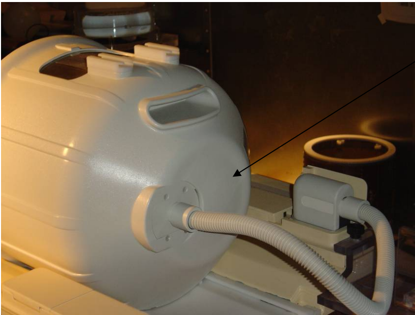
Figure 2. Rear view of TR Brain coil. Note that extensive circuitry is contained in rear backplane of coil.
