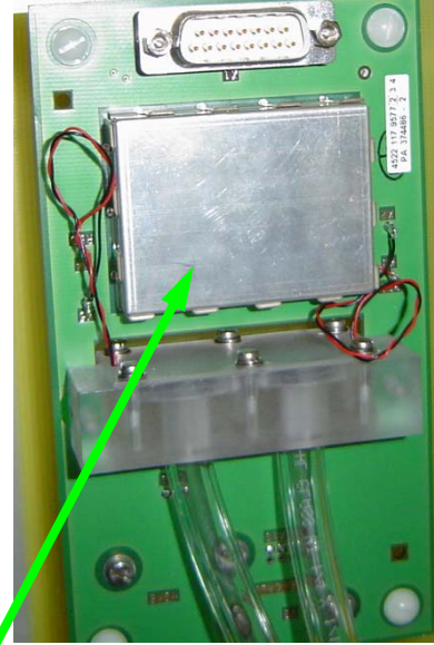
Figure 4: FastTrack Patient Communication (FTCOM) board detail
