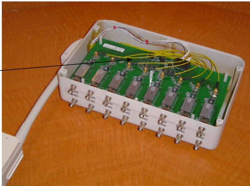
Figure 2 7T Achieva 16Channel interface box, showing circuit boards.
