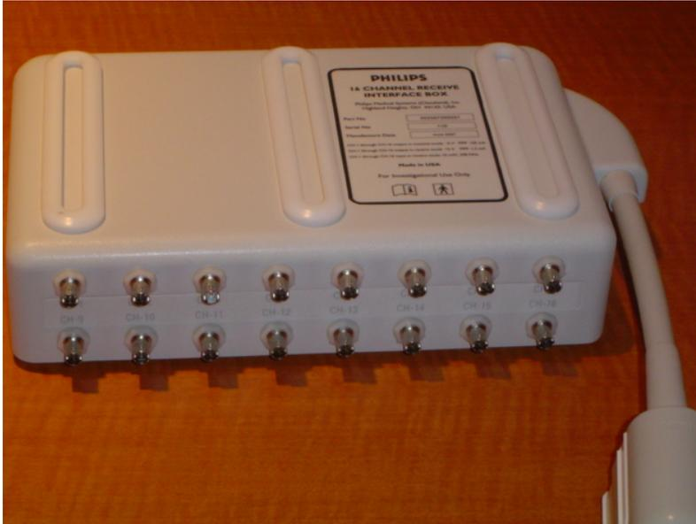
Figure 1. 7T Achieva 16 Channel Interface box.
