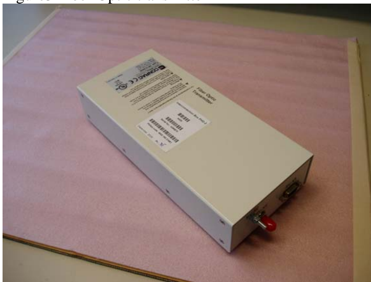
Figure3 Fiber Optic transmitter
