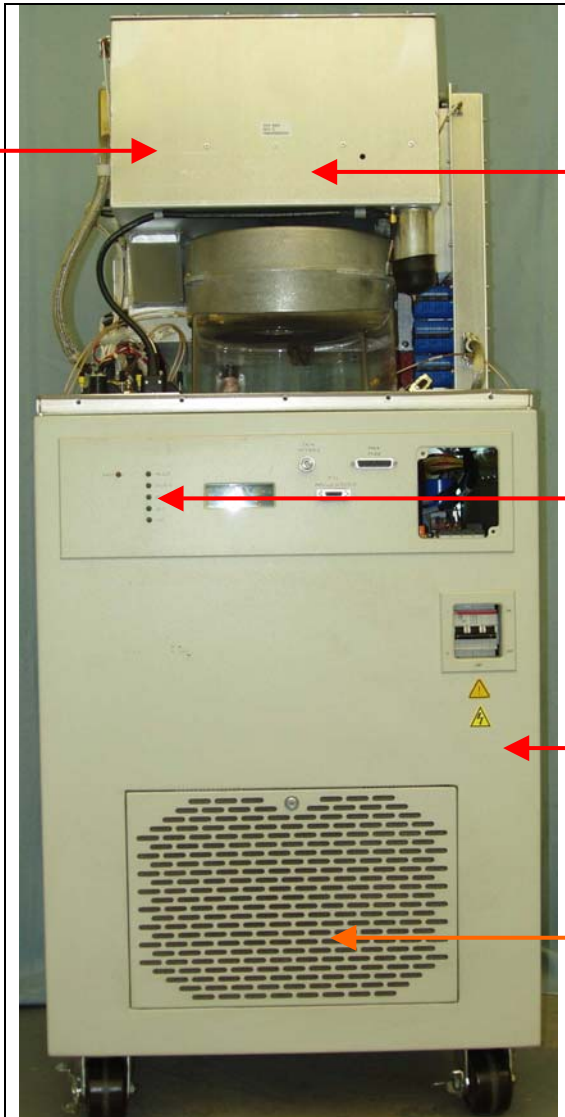
Figure 1: Amplifier Front RF Deck On Top Shown With Covers Removed, Power Supply Below
