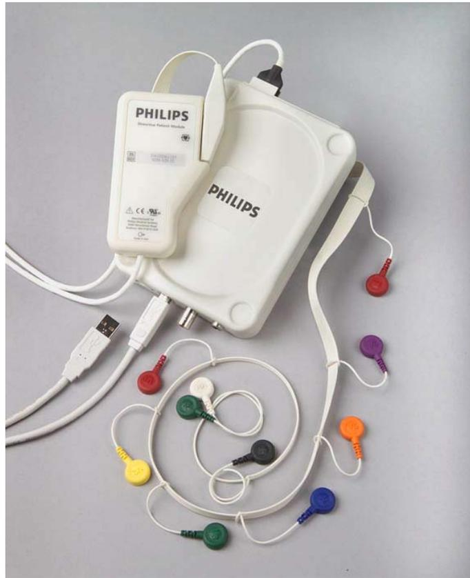
**Direct Wired ECG Module with USB Connector: No battery included**
