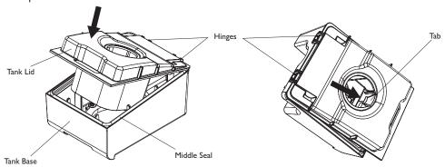
Note: If the lid does not close easily onto the base, separate the two parts, reassemble the tank, and inspect it again.
