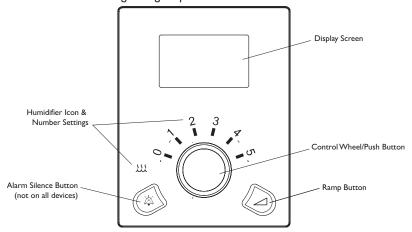
14. Turn the wheel to adjust the Humidifier number to the desired heater plate setting. The settings are 0 (which turns the heater plate off), 1, 2, 3, 4, and 5. The delivered Relative Humidity (RH) shall increase as the setting increases.
