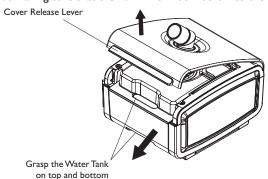
3. Press the tab in the hole on top of the tank in toward the front of the tank. Gently remove the tank lid from the tank base and set aside. Empty any remaining water from the base of the tank.
