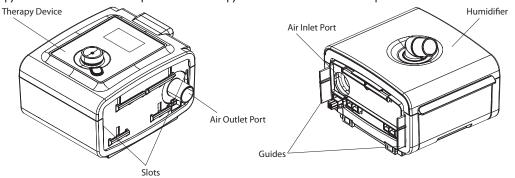
4. Simply press the two units together until they snap into place. Make sure that the therapy device and the humidifier are completely seated against each other.
