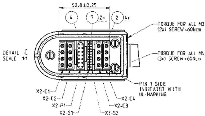
Fig 5: Layout of ODU connector
